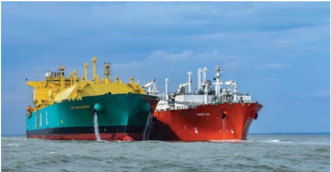
Ship to Ship (STS) LNG Transfer Operation
