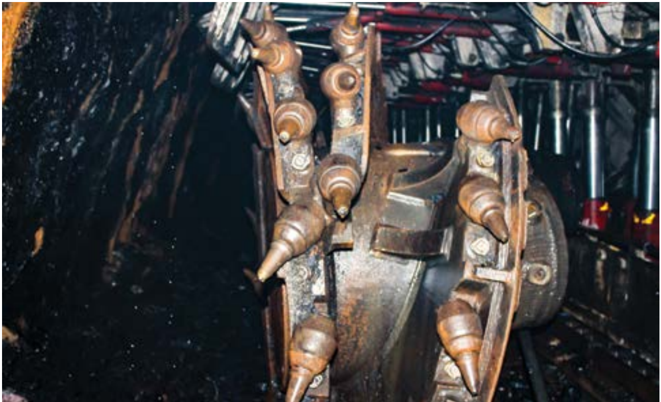
Underground mining with Coal Shearer at BCMCL
